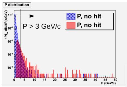
There are tracks with p > 3 GeV/c that do not leave a hit in the detector
