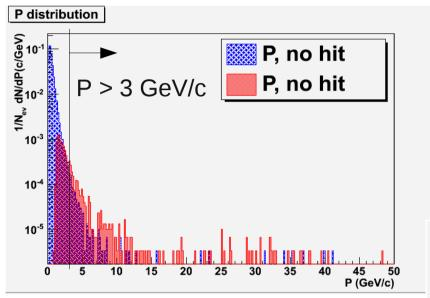
There are tracks with p > 3 GeV/c that do not leave a hit in the detector
