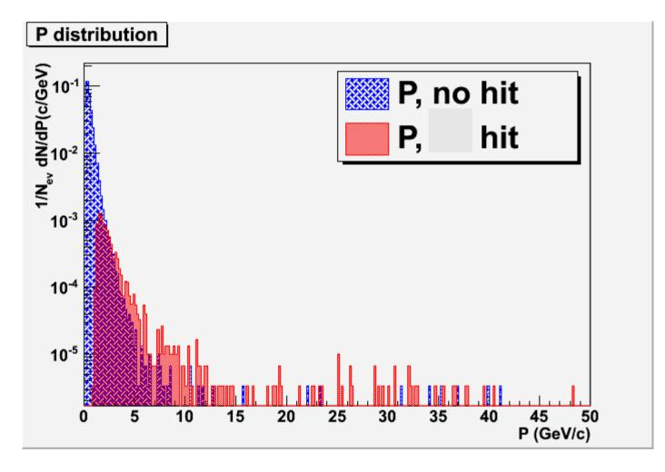
Momentum distribution of tracks inside the module acceptance, based on whether it is a "hit" or "no hit".
